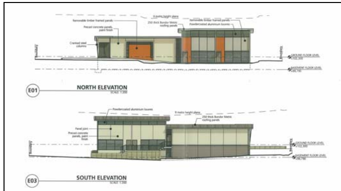
Figure 2 – North & South Substation Elevations
